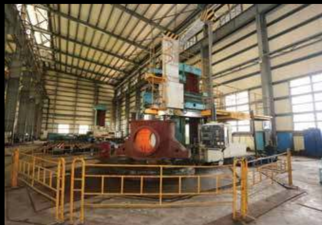
Vertical turning machine SKJ 32-63A Machining capacity: Max.diameter 6300mm Max.length 2500mm
