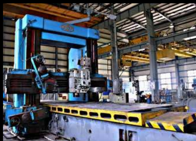
Bed shaper machine HC13T Machining capacity: X/Y/Z 8000 1800 1500mm
