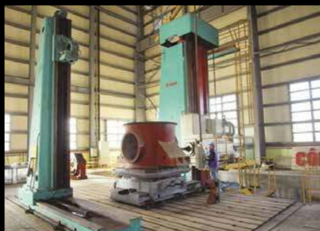
Boring machine W250 Machining capacity: X/Y/Z 7000 2000 4000mm
