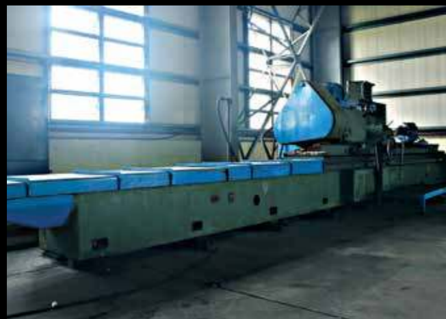
Cylindrical grinding machine 3A172 Machining capacity: Max.diameter 500mm Distance btw center 4000mm
