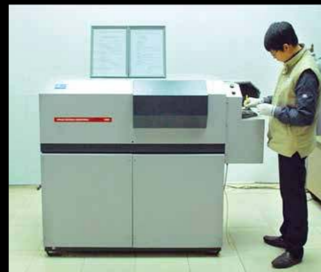
ARG optical emission spectrometer Metals Analyzer of 24 elements( Switzerland)
