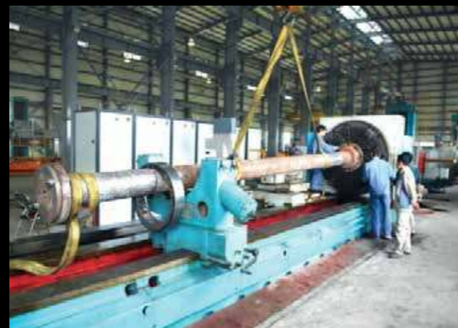
Horizontal turning machine SUT160 Machining capacity: Max.diameter 1600mm Max.length 12000mm
