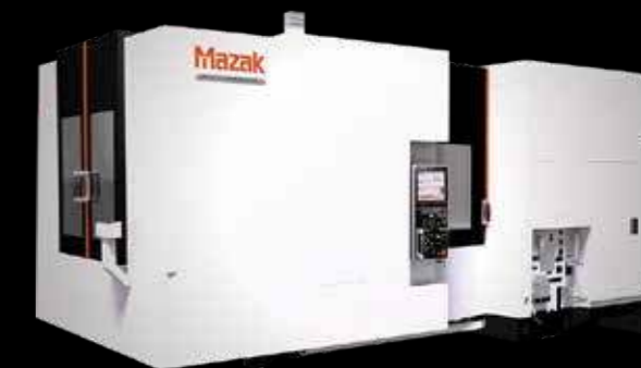
CNC Horizontal machining center with full 360 rotary machining axis Model: HCN-8800 Capacity: X/Y/Z travel 1,400x1,200x1,325mm Origin: Mazak - (New 2018)
