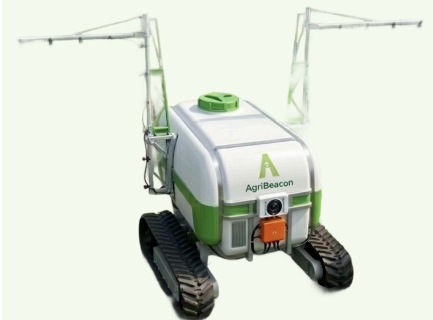
Autonomous multi-purpose robot Self-driving spraying and mowing
